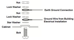
Figure 1-7 Ground Installation
